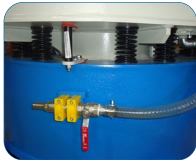
Dirty Water Discharge Pis Su Tahliye
